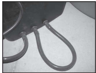
Unused outlets connected with tubing
