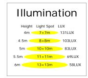
Beam Angle (50% max) 120 DEG Luminous Flux (IES) 3,080 lm Light Efficacy (IES) 77 lm/W **Cutoff Classification** Full-Cutoff
