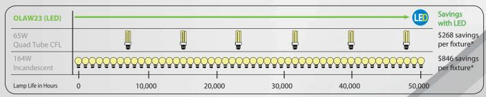
\*Energy savings over the life of the fixture based on difference in input watts @ \$0.12KWh and operating 12 Hours/Day, 365 Days/year. Total savings over life of the fixture is total Energy Savings + Cost of replacement lamps required for traditional source.
