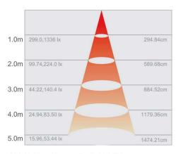
Height Eavg/Emax Angle:111.70deg Diameter
