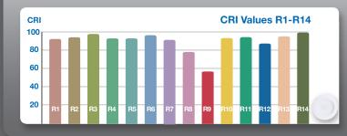
The CRI<sup>SP</sup> SERIES DOWNLIGHT 18W lamp features a typical CRI 90, R9 55 and R13 94, providing crisp and vibrant colors across the whole spectrum. Its exceptional R9-R14 values (R9 & R13) provide redder reds, natural looking skin tones and whiter whites. In addition, this lamp's color temperatures fall within a 4-step Macadam ellipse to ensure minimal color deviation across lamps.
