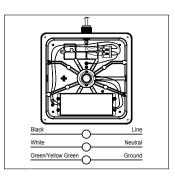
4: Disconnect the wires came from 3/4" hole and connect the wires came from 1/2" conduit with power supply. (White for Neutral, Black for Line, Yellow Green/Green for Ground)
