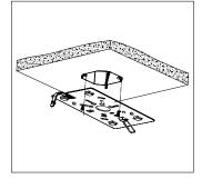
2: Fix the bracket on J-box, and put the wire through the central hole for wiring.
