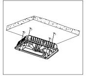
2: Cut off the wires through from 3/4" hole and plug the hole with provided Plug. Drill 4 holes on edge of fixture and fix it on the ceiling with using appropriate screws.
