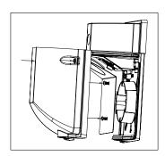
4. Replace the reflector and lens carefully by reversing procedure used to remove it.
