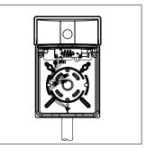
Connect Black for line, White for Neutral and bare wire for Ground to complete the wiring.
