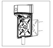
2. Remove the threaded plug from the bottom, Plug the 1/2" conduit into the fixture, konck out 2 screw holes on the back housing and attach the fixture on the wall with proper screws, use the supplied gasket for a weather tight seal.
