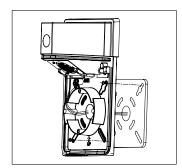
2. Knock out the 2 screw holes and the holes in the center of the back housing, Plug the wires from the J-BOX into the fixture through the center hole, and attach the fixture to the J-box with proper screws. use the supplied gasket for a weather tight seal.
