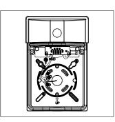
Connect Black for line, White for Neutral and bare wire for Ground to complete the wiring.
