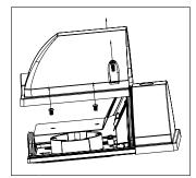
1. Removing the len by loosening the two screws aside the len, removing the reflector by loosening the two screws.
