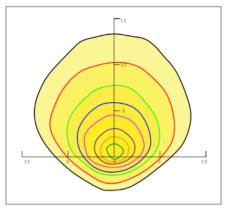
Mounting Hight 4m, 0 Tilt, 50LUX-5LUX
