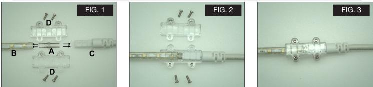
For the power connection you will use the pins that are sharp on one end and blunt on the other. FIG. 1 - Insert pointed end of connector pins (A) into led flat rope light (B) wire holes. *TIP: warming the end of the led flat rope light slightly with a hair dryer will make it more pliable and easier to insert pins.* Make sure pins are inserted as far as possible but be careful not to bend or break connector pins.
