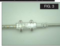
For the power connection you will use the pins that are sharp on one end and blunt on the other.
