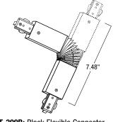
NT-309B: Black Flexible Connector NT-309S: Silver Flexible Connector NT-309W: White Flexible Connector
