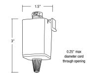
NT-368B: Black Pendant Track Adapter NT-368S: Silver Pendant Track Adapter NT-368W: White Pendant Track Adapter NT-368B/J: Black Pendant Track Adapter (Juno Compatible) NT-368S/J: Silver Pendant Track Adapter (Juno Compatible) NT-368W/J: White Pendant Track Adapter (Juno Compatible)
