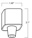
NT-317B: Black Pendant Adapter NT-317S: Silver Pendant Adapter NT-317W: White Pendant Adapter NT-317B/J: Black Pendant Adapter (Juno Compatible) NT-317S/J: Silver Pendant Adapter (Juno Compatible) NT-317W/J: White Pendant Adapter (Juno Compatible)
