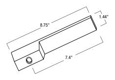
NT-326B: Black Wire Way Cover NT-326S: Silver Wire Way Cover NT-326W: White Wire Way Cover
