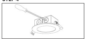
Using a screw driver, carefully remove the knock out as shown above.
