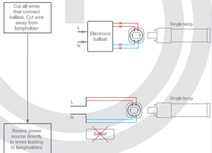
Diagram 3 – Magnetic ballast fixture wiring modification
