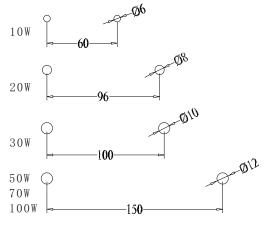
Step 1: Drill holes on installation surface to install M6/M8/M10/M12 bolt
