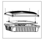
**1:** Remove the lens and metal plate by unscrewing the screws.
