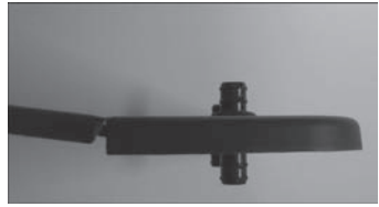
Install straight connectors symmetrically around container and lid
