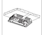
**3:** Remove 1/2" plug from direction you intend to feed conduit.
