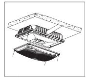
**5:** Replace the metal plate and the lens, make sure no wires are pinched when replacing parts.
