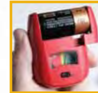
Movable contact arm fits multiple battery sizes
