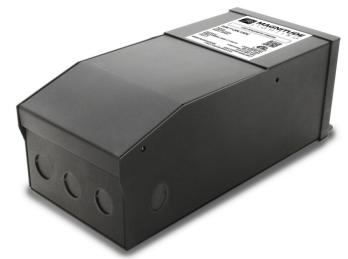
Magnitude's T180L12DC is a multi-output class 2 LED dimmable LED driver. It is equipped with push-to-reset breakers, one on each output, protecting both the load and the driver. Encased in a high-quality NEMA 3R metal case enclosure, that includes 5 knock-outs to enable easy installation. All of our T- Series LED Drivers are dimmable with any standard MLV TRIAC dimmer.
