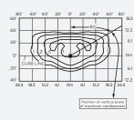
Mounting Height: 25' (7.6m) Initial Delivered Lumens: 3,819 Initial FC at grade
