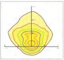
Mounting Hight 4m, 0 Tilt, 50LUX-5LUX
