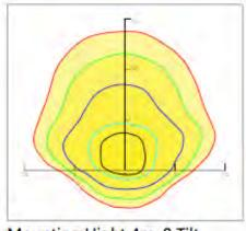
Mounting Hight 4m, 0 Tilt, 50LUX-5LUX
