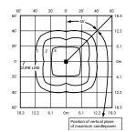
VG-A-\*\*-5W-A-40K-UL Mounting Height: 10' (3.0m) A.F.G. Initial Delivered Lumens: 3,760 Initial FC at grade
