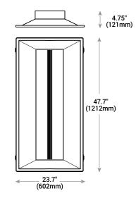
NOTE: Use of Expanded Junction Box will expand the depth to 6.67" and Emergency Backup will expand the depth to 6.30". Use of 347V will increase fixture height by 1.4"
