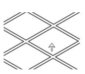
**6.** Remove the ceiling plate then arrange the wire.
