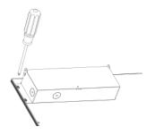
**1.** Remove the screw on both end of theJunction Box, then make the right hole for wire.
