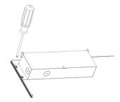
**1.** Remove the screw on both end of the Junction Box, then make the right hole for wire.
