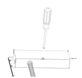
**5.** Fix the cover of the Junction Box then tighten the screw
