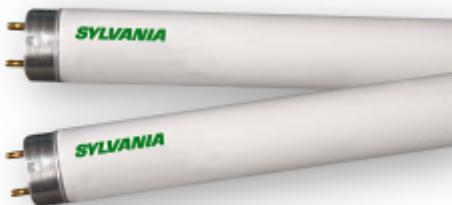
**General Description:** 25W, 48in. MOL, T8 OCTRON Extended Value SUPERSAVER® fluorescent lamp, 3000K color temperature, rare earth phosphor, 83 CRI, suitable for RS or IS operation, ECOLOGIC®.
