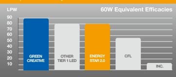
At 89 LPW, this lamp's efficacy is higher than the Tier 1 LED A19 60W replacement industry average and exceeds new ENERGY STAR 2.0 requirements. This energy-saving performance makes this lamp a smart retrofit choice for incandescent and CFL bulbs.
