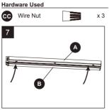
7. Snap the fixture lens cover (B) back onto the fixture plate (A) to complete the installation.
