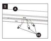
5.Connect the fixture wires to the supply wires -- black to black, white to white, and green to copper/bare.
