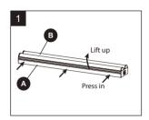
1.Press the bottom frame of the fixture plate (A) inward, in the direction of the arrows, and lift the fixture lens cover (B) with the other hand in the direction indicated.
