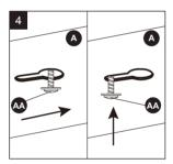
4. Align knockout hole with the supply wire location on the mounting surface and hold the fixture up in its intended location with one hand while marking the location of the two keyhole slots at each end of the fixture plate.
