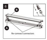
6.Re-connect the connectors between the fixture plate (A) and fixture lens cover (B).
