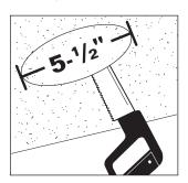
**Step 1:**Using provided stencil, trace cutout lines for housing hole on ceiling. Use saw to make appropriate 5-1/2" cutout.
