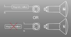
When used with a magnetic ballast, the PL V can function as a plug & play lamp and operate with the existing ballast. If the ballast is not compatible, it can be bypassed and the lamp can run directly off line voltage.
