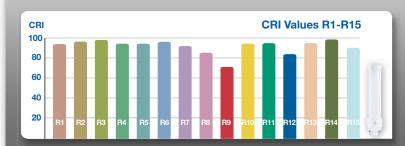
THE CRISP SERIES PL H 10.5W lamp features a typical CRI 90, R9 66 and R13 96, providing crisp and vibrant colors across the whole spectrum. Its exceptional R9-R14 values (R9 & R13) provide redder reds, natural looking skin tones and whiter whites.
