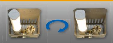
This PL H lamp features a base that can be rotated 310° to fit any socket configuration. After installation simply rotate the lamp to achieve maximum light output.
