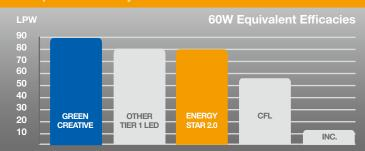
At 89 LPW, this lamp's efficacy is higher than the Tier 1 LED A19 60W replacement industry average and exceeds new ENERGY STAR 2.0 requirements. This energy-saving performance makes this lamp a smart retrofit choice for incandescent and CFL bulbs.
