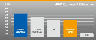
1 LED A19 40W replacement average and exceeds the new ENERGY STAR requirements by upwards of 35%. This energysaving performance makes this lamp a smart retrofit choice for incandescent and CFL bulbs.
