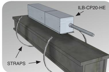
The strapping kit provides (2) straps that run through the mounting tabs of the ILB-CP for securing to a beam or column near the fixture. Overall strap length is 18".
