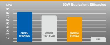
50W replacement industry average and exceeds ENERGY STAR 2.0 requirements. This energy-saving performance makes this lamp a smart retrofit choice for halogen bulbs.
