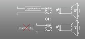
When used with a magnetic ballast, the PL V can function as a plug & play lamp and operate with the existing ballast. If the ballast is not compatible, it can be bypassed and the lamp can run directly off line voltage.
