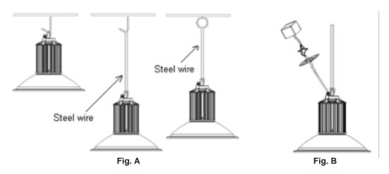
2: Make wire connections, connect the power supply that in the oulet box to the black wire to ( L ), White to ( N ), Green to ( Earth) (see Fig. "B")
