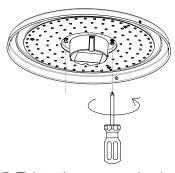
5: Tighten the screws and make sure the lamp is well mounted.
