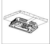
**3:** Remove 1/2" plug from direction you intend to feed conduit.
