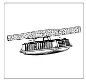
**4:** Slide the Canopy lights into bracket, and secure the screw on side of the light to prevent the light from sliding out from the bracket. Installation done.
