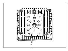
**1:** Loosen the screw on side of the light, removing the bracket from Canopy light by pulling it slightly out, just leaving the ring on bracket. ( See the Step 1 above)
