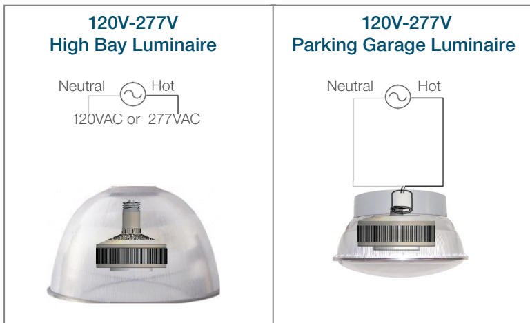
Figure 1: Bypassing the magnetic ballasts; follow steps 1 through 4 in the instructions above to bypass the HID ballast.
