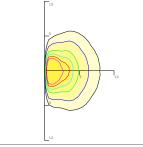
Mounting Hight 3m, 0 Tilt, 50LUX-5LUX
