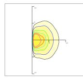
Mounting Hight 3m, 0 Tilt, 50LUX-5LUX
