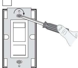
Installation may now be completed by carefully positioning all wires to provide room in wall box for dimmer. Mount dimmer into box with mounting screws supplied. Attach wallplate.
