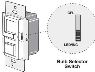
**LED/Incandescent Mode:** The selector switch is pre-set at the factory to this mode. Use this mode for dimmable LED bulbs and incandescent/halogen bulbs. To avoid flickering at the low end of the dimming range you can pre-set the minimum light level. See **OPERATION** to manually program the minimum light level.
