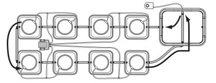
The WaterFarm 8-Pack circulating pump pulls nutrient solution from the first individual reservoir and mixes with the nutrient solution in the controller, then flows out through the opposite individual reservoir because of the difference in the level of the nutrient solution. The entire system will cycle in approximately 4 hours end effectively maintain a consistent nutrient in all of the individual reservoirs.
