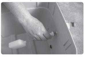
Secure the Float Valve from the outside of the Controller with the brass nut. Coat the remaining threads with the Pipe Thread Compound and screw on the brass 1/2" barbed hose fitting.
