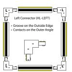
Using a right connector, the track would run with the groove along the inside
