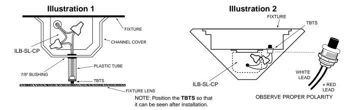
Linear Fixture – Select a convenient location on the fixture so the **TBTS** can be seen after installation. Allow for proper clearance inside the fixture and drill or punch a 1/2" hole. Remove the nut from the **TBTS**. Push the **TBTS** housing into the 1/2" hole and secure with the nut. Connect the LED wires from the unit to the **TBTS** (Red/Black or Red w/tag to Red, White/Red to White). Refer to *Illustration 2*.
