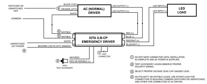
CONNECT UNSWITCHED POWER. IF A SINGLE BUILDING COMMON IS PRESENT, CONNECT THE WHITE WIRE TO THE COMMON. IF A SEPERATE UNSWITCHED CONDUCTOR FEED IS PRESENT, CONNECT THE WHITE LEAD TO THE COMMON FROM THE
