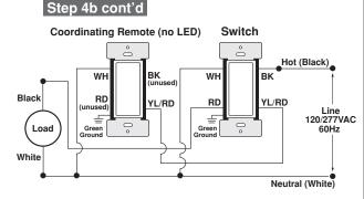
NOTE: The switch must be installed in a wall box that has a Line Hot connection. The coordinating remote must be installed in a wall box with a Load connection and a Neutral connection. A Neutral wire to the coordinating remote needs to be added as shown. If you are unsure about any part of these instructions, consult an electrician.
