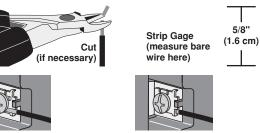
Side Wire Connection **Back Wire Connection** Side wire terminals accept #14-12 Back wire openings accept #14-12 AWG solid copper wire only. AWG solid copper wire only.
