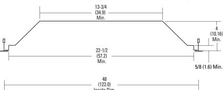
Relight assemblies are designed to fit most recessed fixtures mounted in T-grid installations. For surface mounted fixtures or for fixtures mounted in ceiling types other than T-grids, consult factory before ordering.
