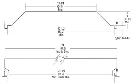
Relight assemblies are designed to fit most recessed fixtures mounted in T-grid installations. For surface mounted fixtures or for fixtures mounted in ceiling types other than T-grids, consult factory before ordering.
